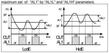
LHAb = ABSOLUTE BAND ALARM: The alarm is activated when the process value goes under the alarm threshold set on parameter "AL1L" or goes higher than the alarm threshold set on parameter "AL1H" and will be deactivated when it goes below the value [AL1H - HAL1] or when it goes above the value [AL1L + HAL1].
