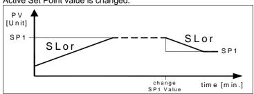
If it is desired an automatic cycle from the power on instead it is necessary to program the par. "nSP" = 2, to program the two Set Point values "SP1" and "SP2" and naturally to program the par. "SLor". "dur.t" and "SLoF" with the desired values.
