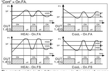
The control works in the following way : in the case of reverse action, or heating ("FunC"=HEAt), it deactivates the output, when the process value reaches [SP + HSEt] in case of symmetrical hysteresis, or [SP] in case of asymmetrical hysteresis and is then activated again when the process value goes below value [SP -HSEt1.
