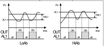
**LodE** = DEVIATION LOW ALARM: The alarm is activated when the process value goes below the value [SP + AL1] and will be deactivated when it goes above the value [SP + AL1 + HAL1]. With this mode is possible to program the minimum and the maximum set of "AL1" by "AL1L" and "AL1H" parameters.
