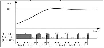
In order to obtain good stability of the process variable, in the event All the parameters referring to Neutral Zone ON/OFF control are of fast processes, the cycle time "tcr1" has to have a low value with a very frequent intervention of the control output.
