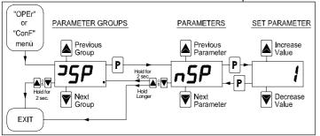
**ATTENTION:** The instrument is programmed in factory with all the parameters, to exception of the Set Point "SP1" (and 2,3,4), programmable in the menù "ConF" to the purpose to prevent wrong accidental programming from non experienced consumers.
