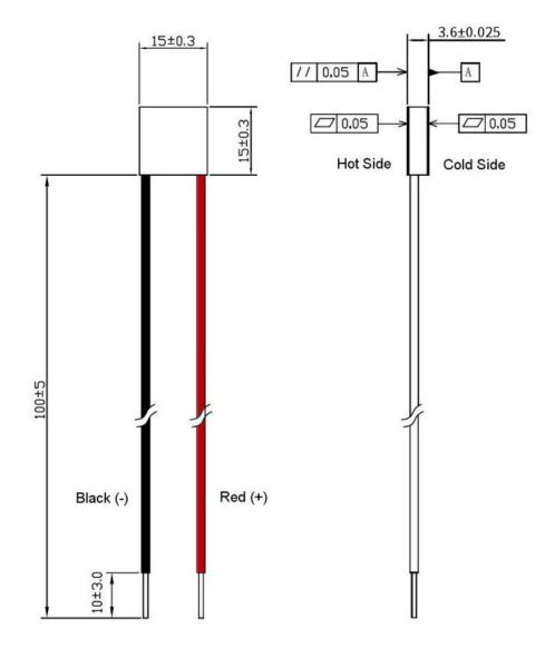
$I_{max}$  = 3.9 Amps ( $I_{max}$  is the maximum current at  $\Delta T_{max}$ )
