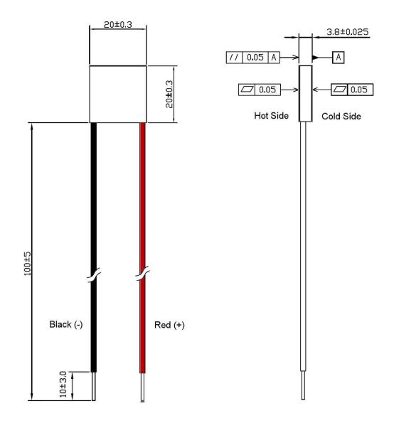
$I_{max}$  = 3.0 Amps ( $I_{max}$  is the maximum current at  $\Delta T_{max}$ )
